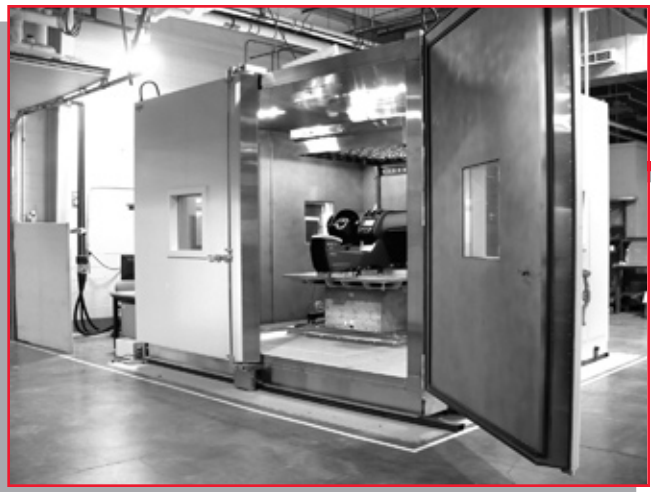
FIG. 5—Environmental chamber with cockpit module on 6DOF actuator system.
